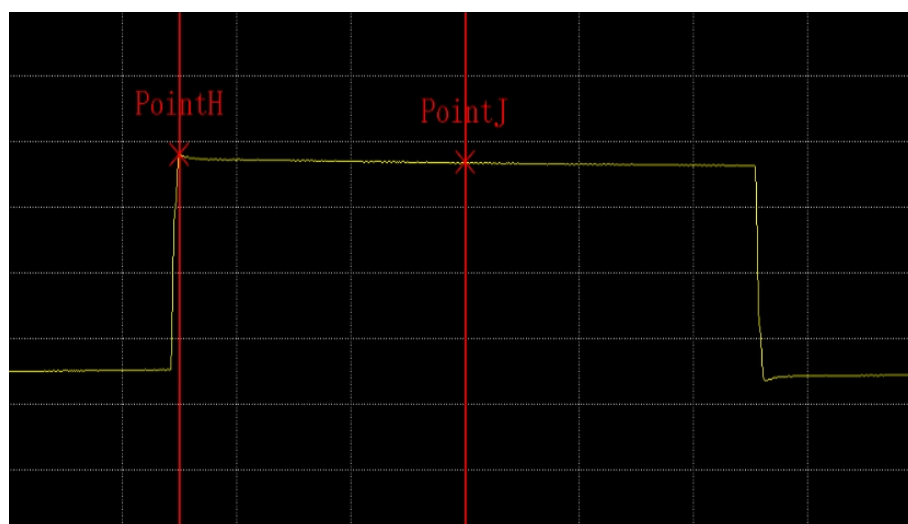
Figure 4.13 Max. Output Droop (Point H and Point J)
